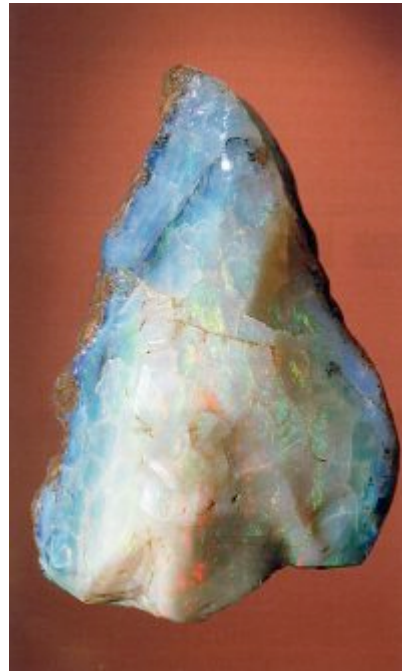
Fig. 9. 'Hungarian' opal rough of 594g (13x7x7cm) from the Naturalhistorisches Museum, Wien. This type 1 opal displays body tones ranging from white opal (N9) to dark blue opal (N5).
